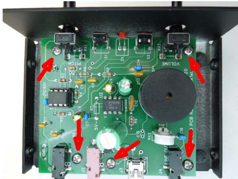
Figure 13 – Attach PCB to enclosure base with five screws
