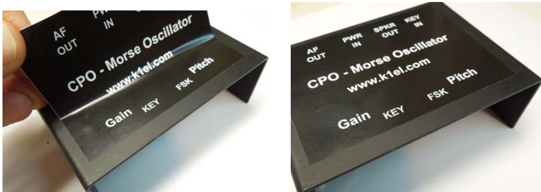
Figure 12 – Carefully align and attach top sticker
