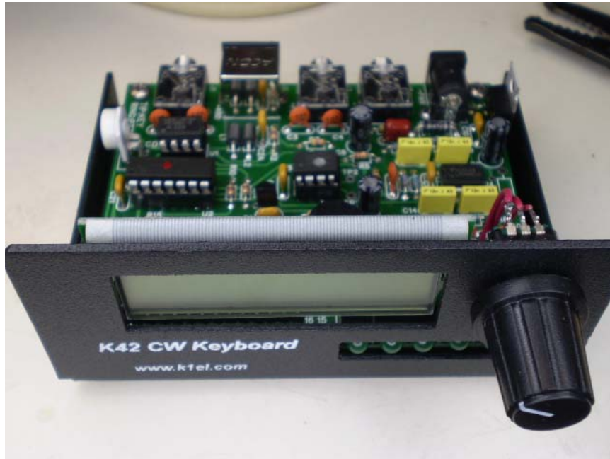
Completed base assembly front view
