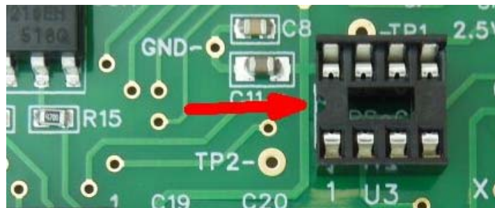
Figure 3 – U3 Socket installed, red arrow indicates socket notch location
