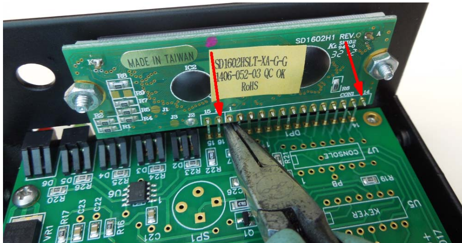
Figure 15 – Gently adjust header for equal pin alignment
