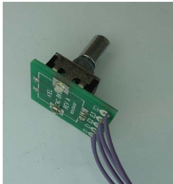
Figure 22 - Encoder on encoder PCB
