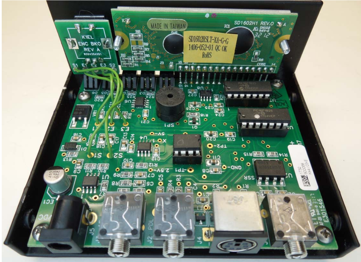
Figure 24 – Rear view with encoder and display in place
