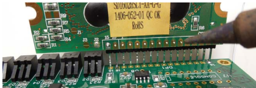
Figure 17a – Solder remaining connections on display
