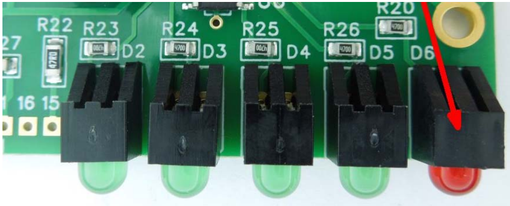
Figure 7 - LEDs installed, note RED LED is on the right side !
