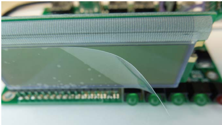
Figure 23 - Don't forget this step or the display will look foggy !
