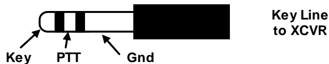
Figure 26 – Key Output Connector
