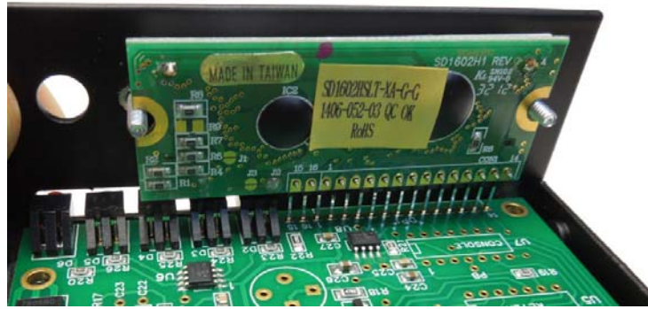
Figure 12 – Subassembly in place on K44 enclosure base
