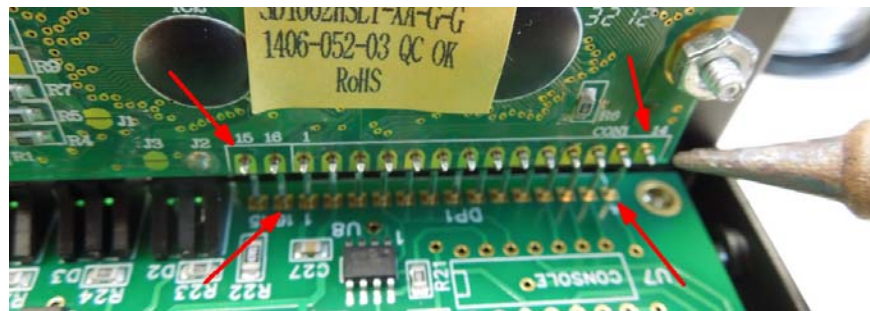
Figure 16 – Solder four places to fix display alignment
