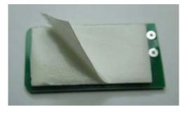
Figure 6 – Remove foam tape paper film
