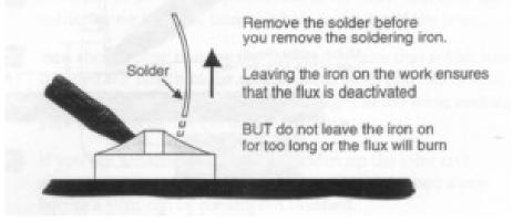
Fig C3 - Remove the solder
