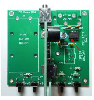
Figure 22 – PSbase components installed
