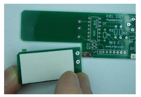
Bend the paddle section to break it free. Trim off separator remnant and use sandpaper to remove burs.
