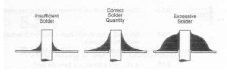
Fig. C4 - Solder quantity comparison
