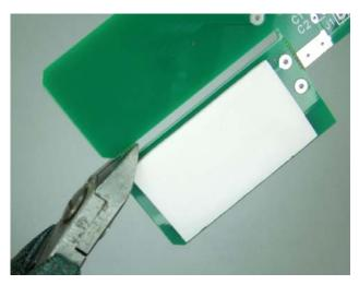
Figure 3 - Cut paddle separator
