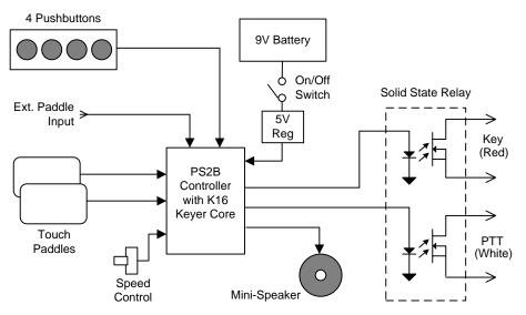
Figure 1 – PaddleStick PS2B Block Diagram
