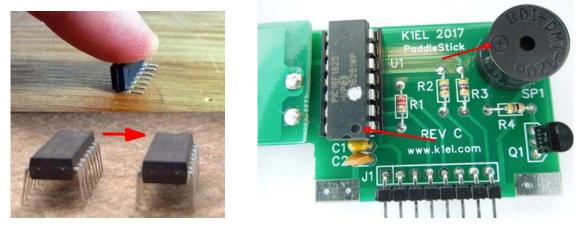
Figure 14 – Straighten leads on U1, then install speaker, transistor Q1, and U1.
