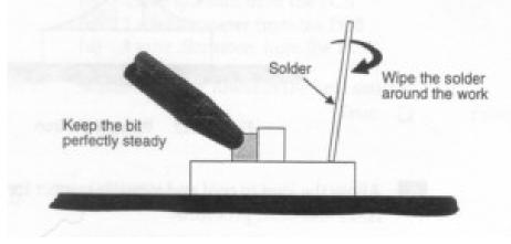
Fig. C2 - Spread solder around the work
