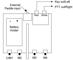
Figure 28 - PaddleStick Connection Diagram
