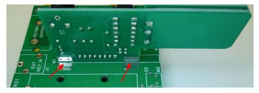
Figure 17 - Red arrow indicate solder bonding zones
