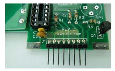
Figure 12 – 8 pin header in place
