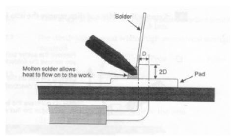
Fig. C1 - Form a heat bridge
