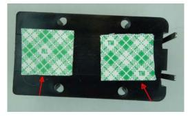
Figure 23 – Foam tape in place on battery holder
