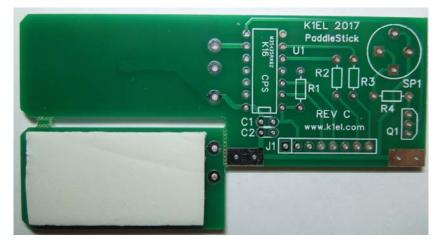
Figure 2 - PaddleStick PC Board before assembly
