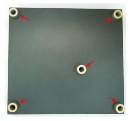
Figure 27 – Spacers placed on top of metal base
