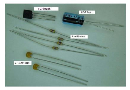
Figure 20 – PSbase components, phase 1
