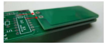
Figure 7 – Assemble paddle halves
