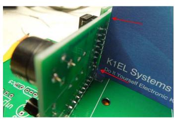
Figure 16 - Verify that the PS is at a right angle to the PSB
