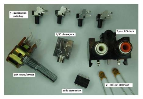
Figure 21 – PSbase components, phase 2 (DIP8 socket not shown)
