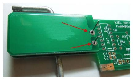
Figure 8 – Insert resistor lead scraps through holes in both boards
