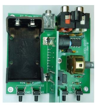
Figure 24 - Completed PSB board assembly
