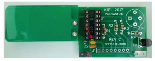
Figure 11 - Install socket, R's, C's, and Q1
