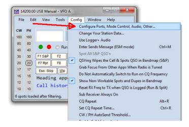
This brings up the Configurer dialog box. This is where devices attached to N1MM+ are set up. For this example we will set up a WinKeyer device on COM2.
