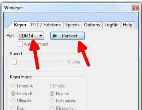
Now Connect changes to Connected and items in the dialog box are no longer grayed out. If you click Auto-connect, DM780 will connect to Winkeyer automatically on startup.
