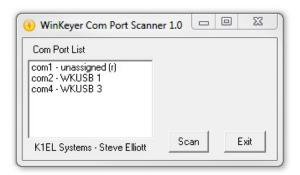
After you have installed WKscan, start it up and you will see the dialog box shown at left. Click Scan and WKscan will display all of the serial ports found on the system. The ports will either be identified as unassigned, in use, or attached to a WK device. In this example we have a WinKeyer1 device on COM2 and a WinKeyer3 device on COM4. Yes, multiple WKs can be operated from a single PC using two applications.
