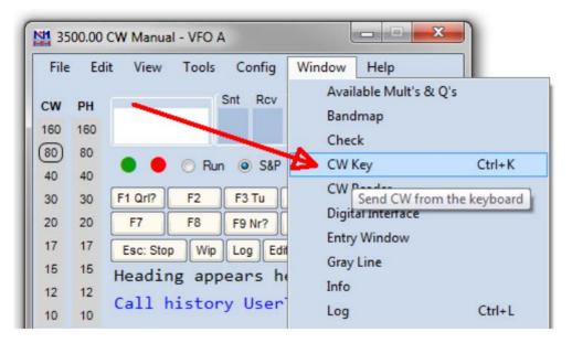
The CW keyboard window is now displayed and you can type into it to send letters to WKmini. Note that when the Send CW window is up, the main N1MM+ dialog box is disabled. For a final test, turn the speed pot and you should see the CW Speed display in the main N1MM+ dialog box change. (This assumes that the speed pot has been enabled in the Winkey configuration dialog box)
