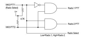
The PTT outputs on WKMINI are open collector so pull up resistors are required to generate logic high and low conditions. PTT1 will be logic zero when radio 1 is selected and logic one when radio 2 is selected.
