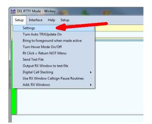
Click *Setup->Settings* to bring up the Digital Setup Window, click on the Message Setup tab and then select "Other, TinyFSK, Winkey" from the drop down menu.
