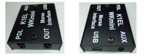
There are four connectors on WKmini, PDL and OUT on the left with AUX and USB on the right.
