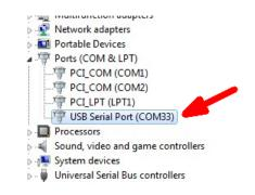
WK's port will be listed under Ports (com & LPT). If more than one USB Serial Port is listed disconnect WKmini's USB cable and see which device entry is removed. Now you know WKmini's com port assignment. In this example it's 33 which may not work with all WK apps. To change it, double click WKmini's USB Serial port entry to view the port properties dialog box.
