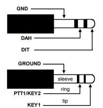
There are four connectors on WKmini, two on the left side and two on the right, The left facing connectors are labeled PDL and OUT. The PDL connector is an 1/8" stereo jack which accepts paddleset input. The paddle can be an iambic or single lever, a bug is not acceptable. The paddle inputs are activated when switched to ground (GND)
