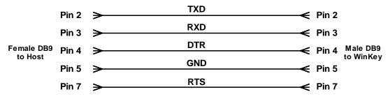
Figure 5 – WinKey RS232 Interface Cable Schematic
