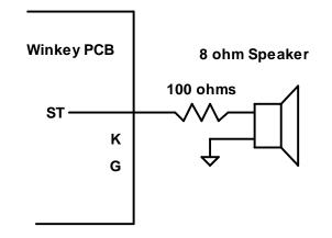
Figure 12 - Sidetone Connection for WinKey PCB
