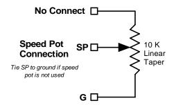
Figure 2 – Speed pot Connection
