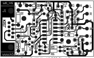
Figure 7 - WinKey V6 PCB Check Plot
