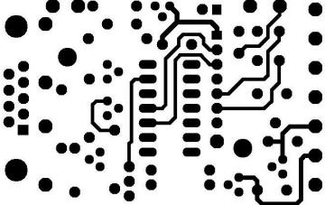
Figure 9 - WinKey V6 PCB Top Solder Side
