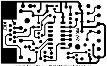
Figure 10 - WinKey V6 PCB Bottom Solder Side
