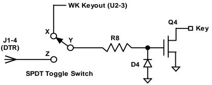
Figure 11 – Key Out Source Switching Option
