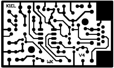
Figure 7 - WinKey PCB Solder Side
