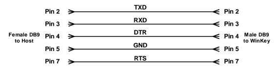
Figure 3 – WinKey RS232 Interface Cable Schematic
