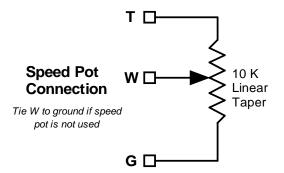
Figure 2 – Speed pot Connection
