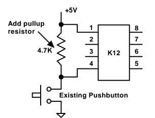
Simply solder a 4.7K 1/4 or 1/16 watt resistor between ppin pads 1 and 4 on the bottom (solder) side of the PC board.
