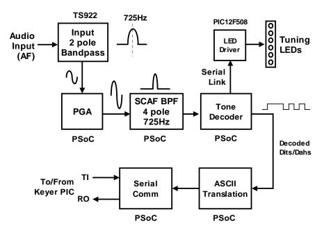
Figure 8 - K44 CW Reader Block Diagram
