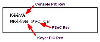
Figure 2 – Typical K44 Power On Screen
