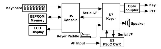
Figure 6 - K44 CW Keyboard Block Diagram
