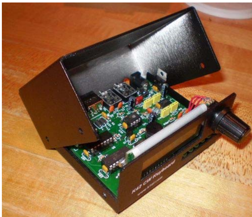
Figure 30 – Fold top cover into place
