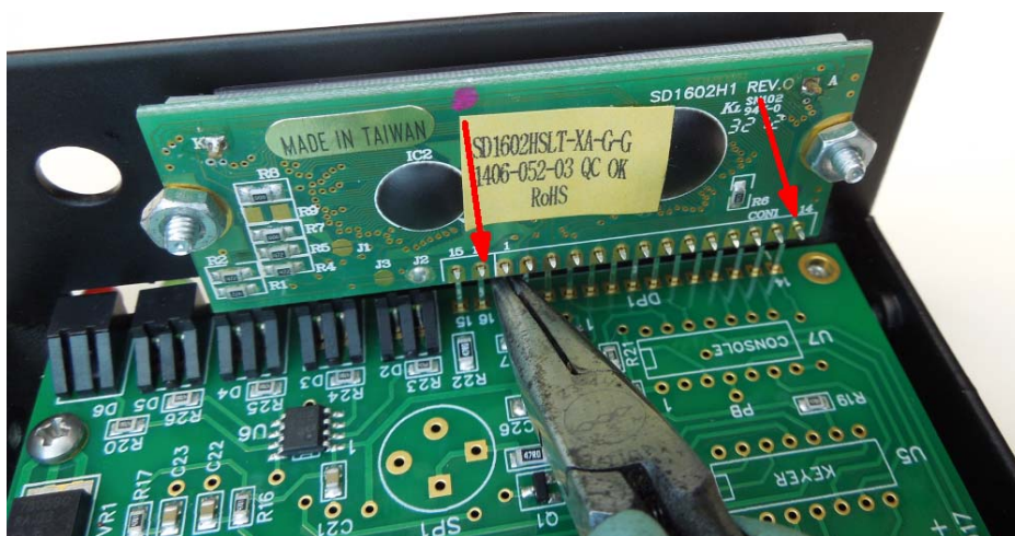
Figure 15 – Gently adjust header for equal pin alignment
