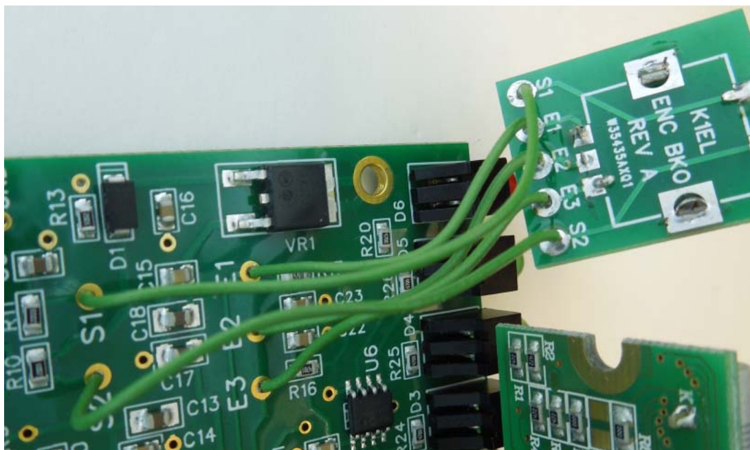
Figure 22 - Encoder PCB attached to main K44 PCB
