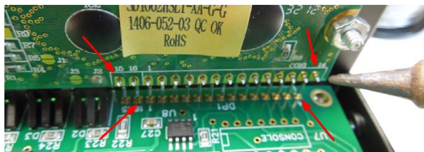
Figure 16 – Solder four places to fix display alignment
