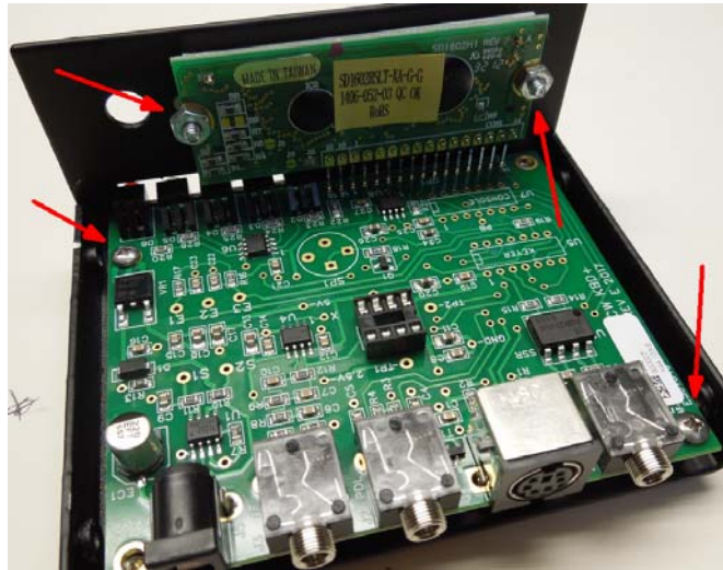
Figure 12 – Add 4-40 nuts and screws to hold subassembly in place
