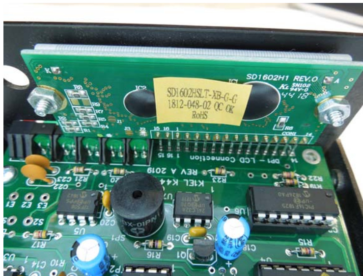
Figure 13 – Close up of display fixed to front panel ( DO NOT OVER-TIGHTEN DISPLAY NUTS !! )
