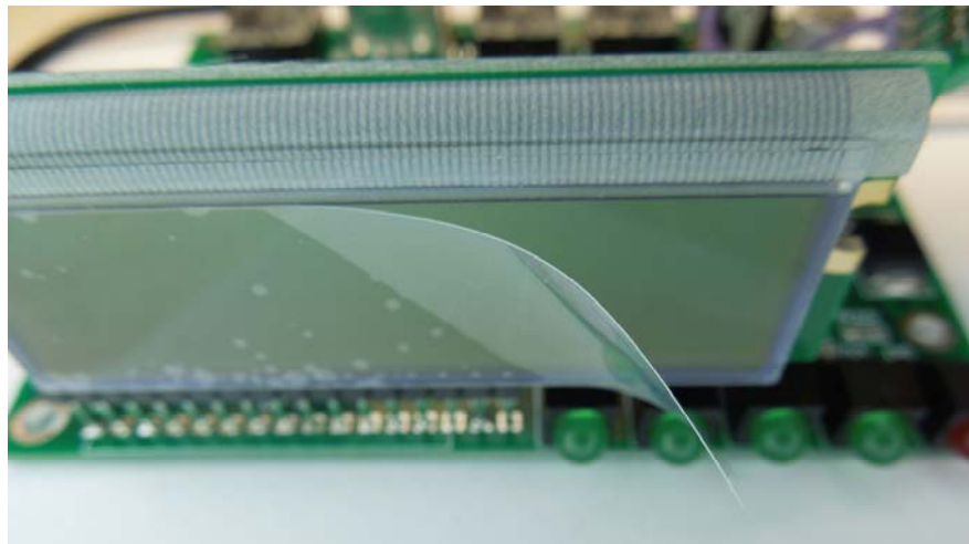
Figure 23 - Don't forget this step or the display will appear foggy !
