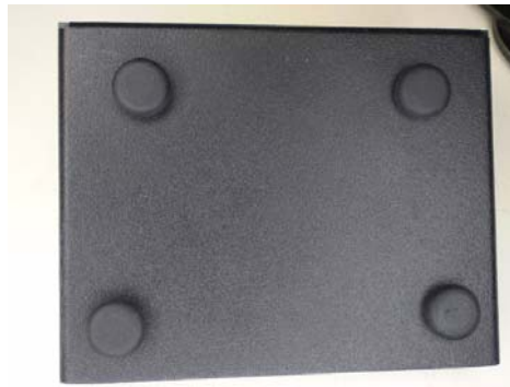
Figure 8 - Rubber feet in place on bottom half of enclosure
