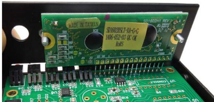
Figure 8 – Subassembly in place on K44 enclosure base
