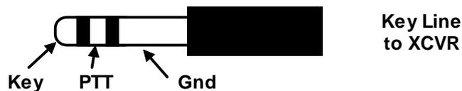
Figure 24 – Key Output Connector
