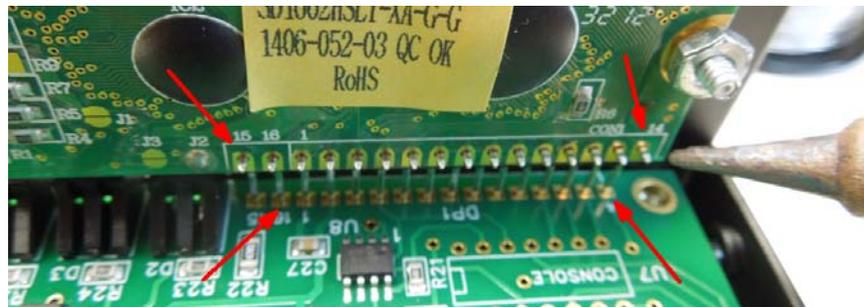
Figure 12 – Solder four places to fix display alignment
