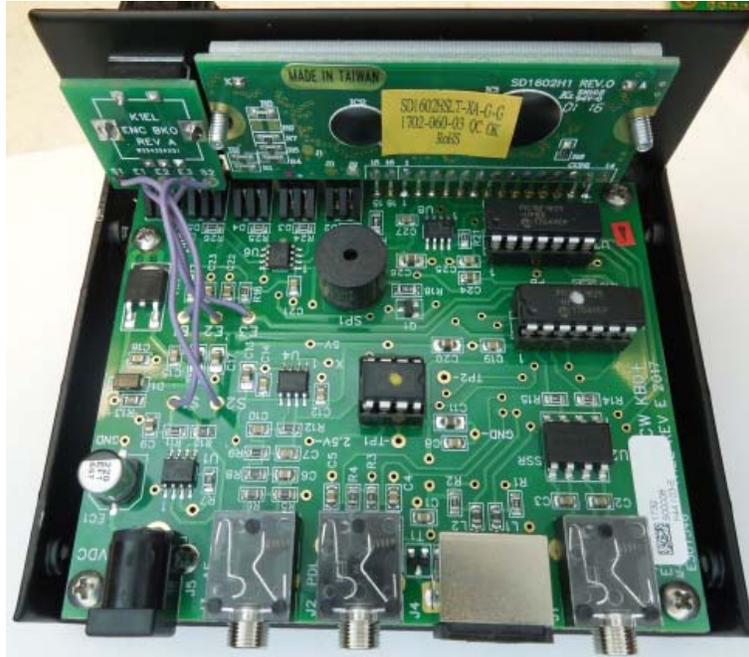
Figure 1 – Assembled K44
