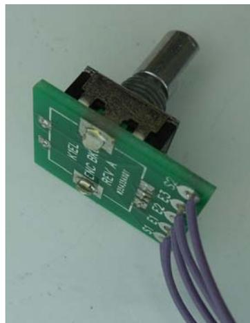
Figure 18 - Encoder on encoder PCB
