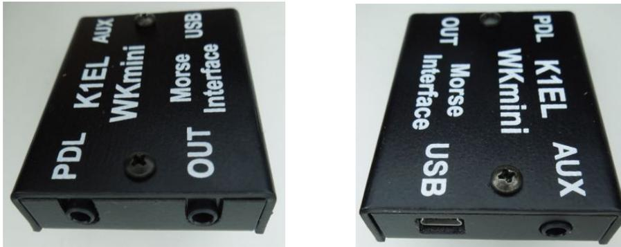
There are four connectors on WKmini, PDL and OUT on the left with AUX and USB on the right.
