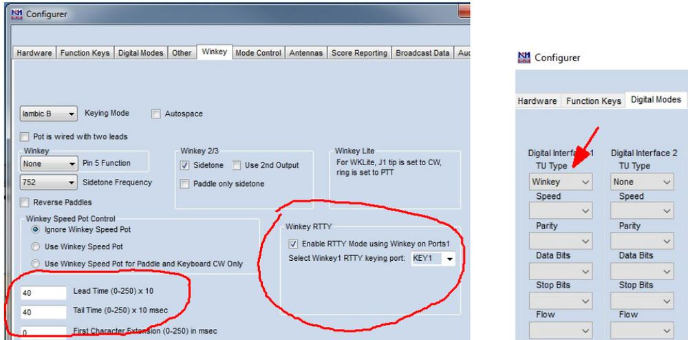
Click on Enable RTTY and then set a delay in both Lead Time and Tail Time; 40 mSec in each is a good starting point. Now click on the Configurer Digital Modes tab and in the left most drop down, select Winkey. Now close the Configurer and go back to the main N1MM+ window. From there we will open up the digital interface window:
