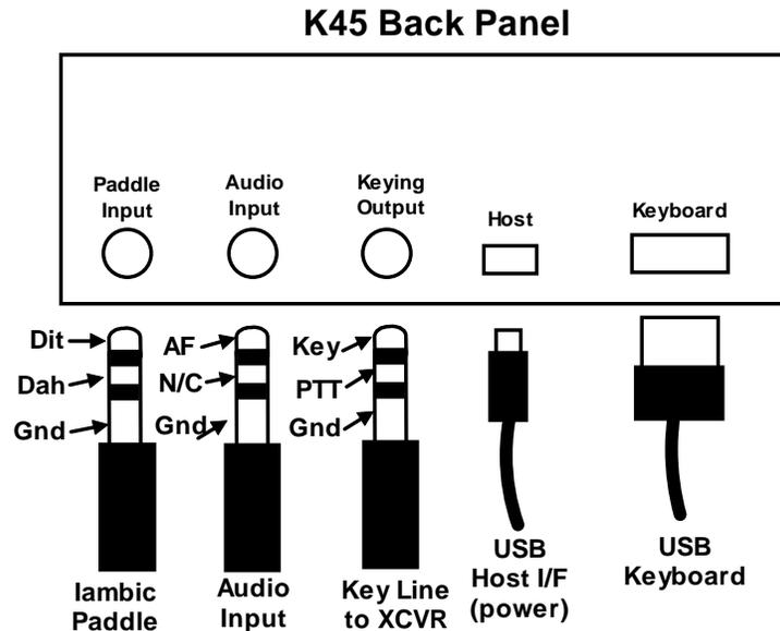
Figure 31 - K45 CW Keyboard Hookup Diagram
