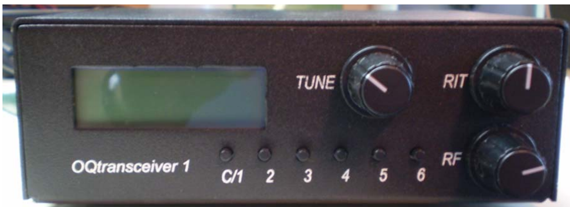
Completed OQ transceiver
